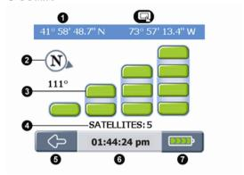
From any navigation screen, tap the GPS icon to display the GPS Status screen. This screen provides a visual representation of the GPS information being received.
